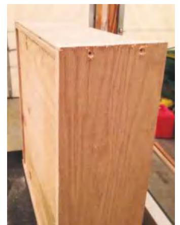
STEP 15. Next, cut and edge the left and right shelves with finishing trim, then, measure and cut the drawer fronts to the size of the openings. I opted for two drawers at the bottom and left the top open for a digital box and/or DVD player
